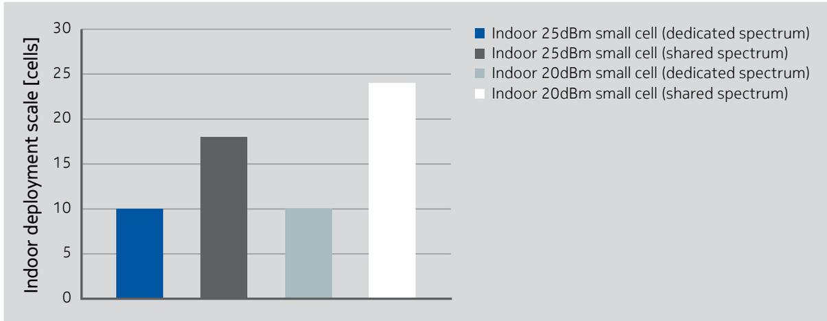
Figure 6: Example of dense indoor deployment per 10,000 m<sup>2</sup> with expected 2020 traffic levels.
