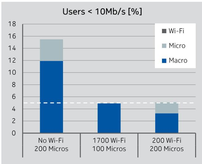
Figure 3: Example of indoor offload via Wi-Fi cells in a dense urban area with 20 macro sites and 200 micro cells.
