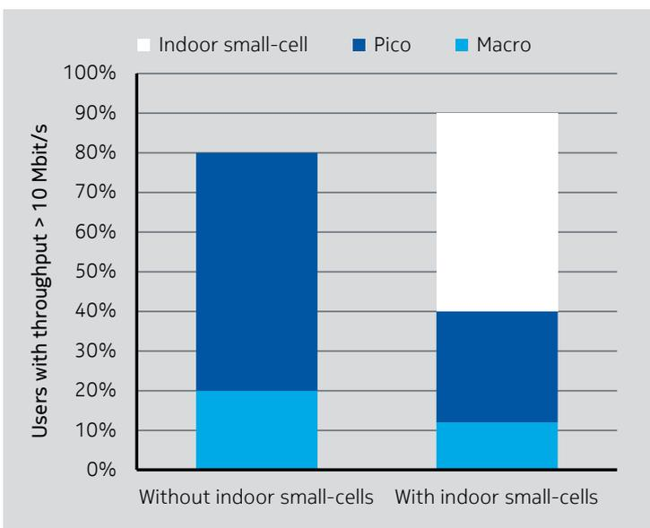
Figure 5: Example of outdoor and indoor small cell (4G/LTE and Wi-Fi 802.11n/ac) coverage probability performance under a typical dense urban deployment scenario as expected in 2020.
