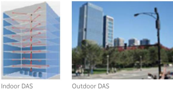
Figure 2: Distributed Antenna Systems (DAS)
