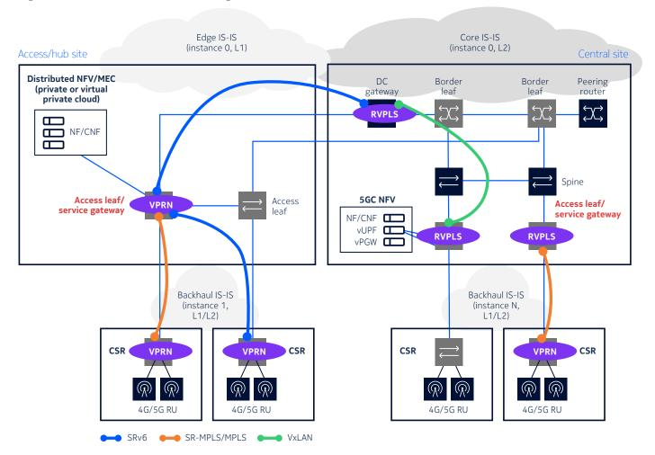
Network operators have successfully deployed SR-MPLS in the telco cloud edge within a private network data center. SRv6 is a strong alternative for implementations in private network data centers, and an even stronger alternative within the public cloud, where an IP tunneling mechanism is needed.
