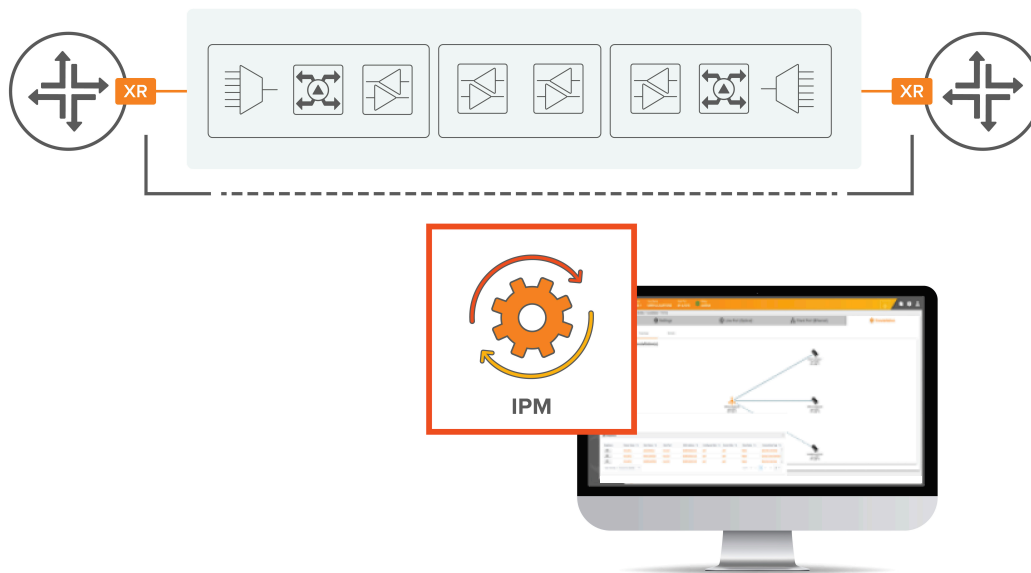
Figure 1: Nokia's Intelligent Pluggables Manager offers holistic transport management of intelligent coherent pluggable optics hosted in networking platforms such as routers, switches, compute servers, or radio units
