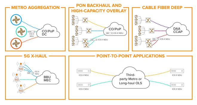
Figure 2: ICE-X network access and aggregation applications
