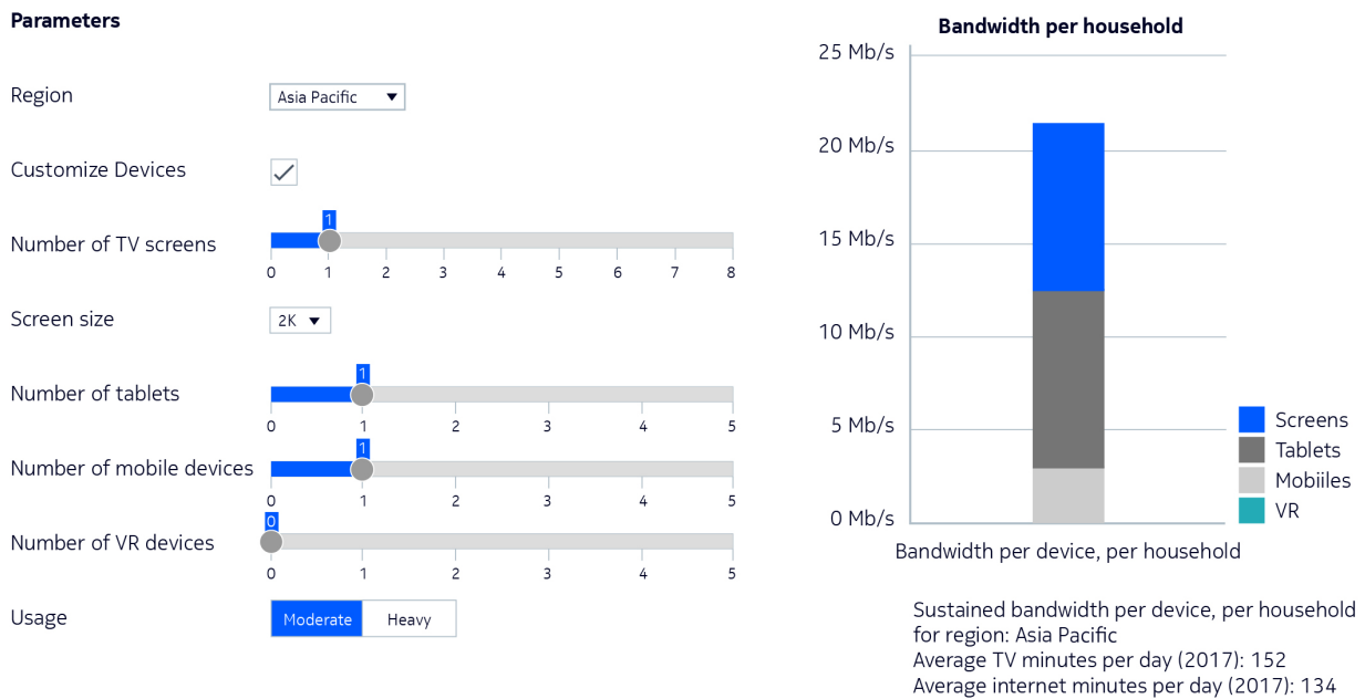
Figure 4: Bandwidth modelling Fixed Wireless Access (FWA) / developed bell labs
